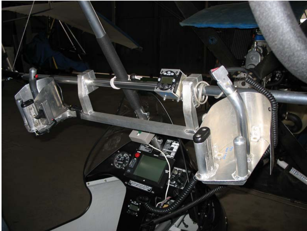
Figure 12 – Control Bar on XT912
