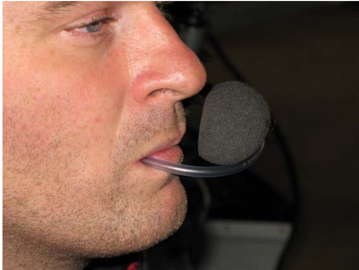
Figure 1 & 2 – Puff/suck tube for steering control
