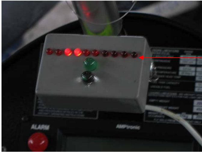
Figure 8 & 9 – LED position indicator
